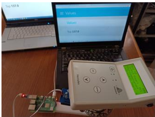
Fig.13 Complete inertia system with sensor, gray code and connection with raspberry and laptop.
